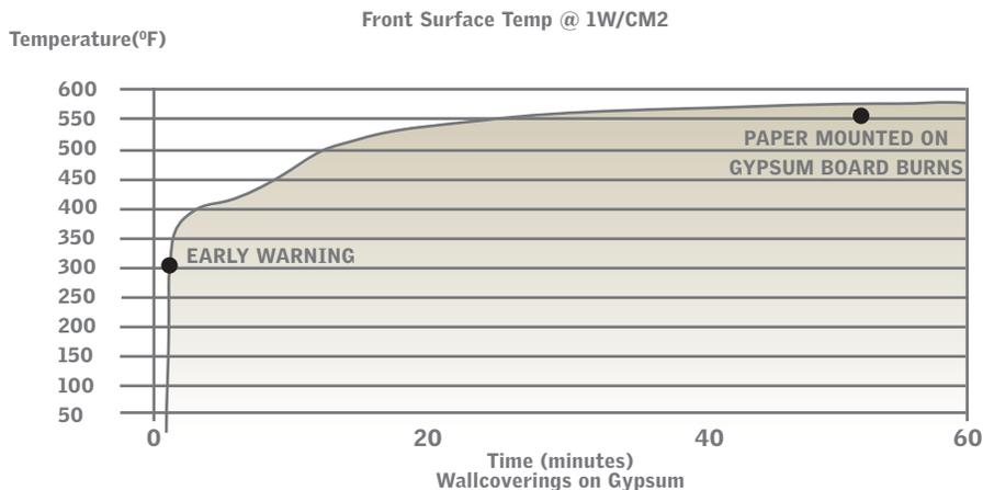
This chart shows how Early Warning Effect® formulation acts over a given time period with a steady flow of heat. This is not typical of a fire environment as no two situations are alike. However, it does give you some idea of how EWE can work.
